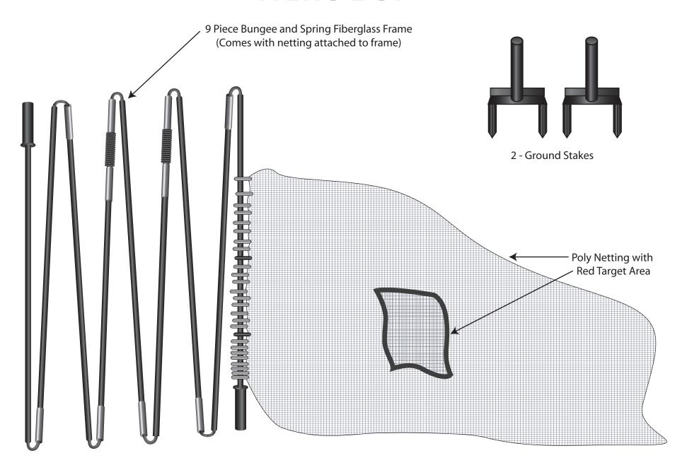
STEP 1 Tap or push both Ground Stakes into ground 7 feet apart. (Caution: Do not pound on the stake top. Damage could prevent frame from inserting properly) — 7 feet STEP 2 Assemble Fiberglass Frame by inserting each pole end into the adjoining metal joint. (Note: Make sure not to pinch the bungee cord)
