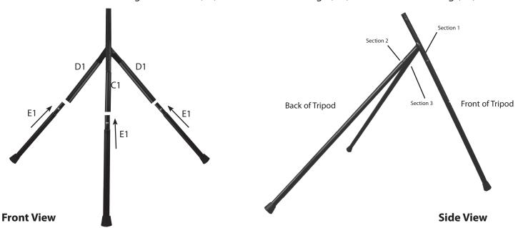
**STEP 3:** Attaching Machine to Tripod
