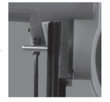
**B:** Slide the Machine Housing (A) close to the Tripod (B), making sure the Tripod (B) fits inside the Pole Clamp (I).
