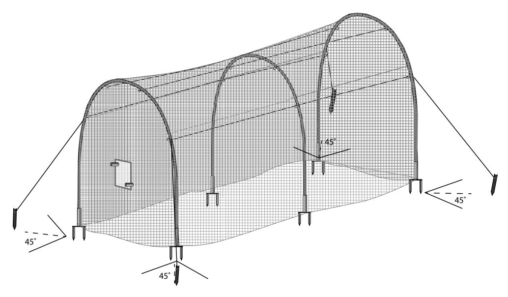
STEP 6: With the Double Ropes With Stake (Part K), find the square net hole nearest to the fiberglass rod fitting shown below and tie the rope to the metal fiberglass rod fitting. **Do not tie the rope to the net.**
