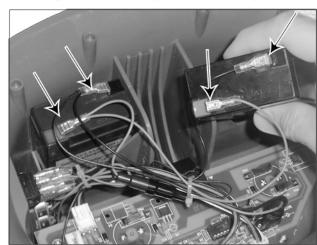
For single battery installation use one set of battery wires.
