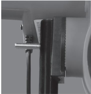
**B:** Slide the Machine Housing (A) close to the Tripod (B), making sure the Tripod fits inside the Pole Clamp.
