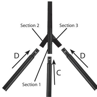
**STEP 2:** Insert Bottom Leg Assemblies (E) in to Middle Back Legs (D) and Middle Front Leg (C)
