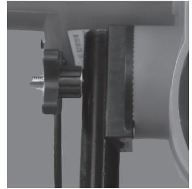
**C:** Slide Flat Washer (1st) and Lock Washer (2nd) on to the Long Bolt, then tighten the Knob on to Long Bolt until machine is placed in the desired pitching position.
