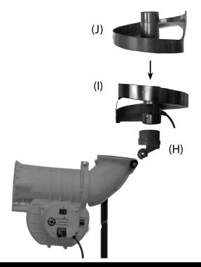
Attach Part H Feeder Port To Housing With Provided Hardware.
