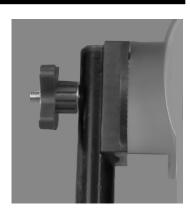
Side Flat Washer (1st) and Lock Washer (2nd) on to the Long Bolt, then tighten the Knob on to Long Bolt until machine is placed in the desired pitching position.
